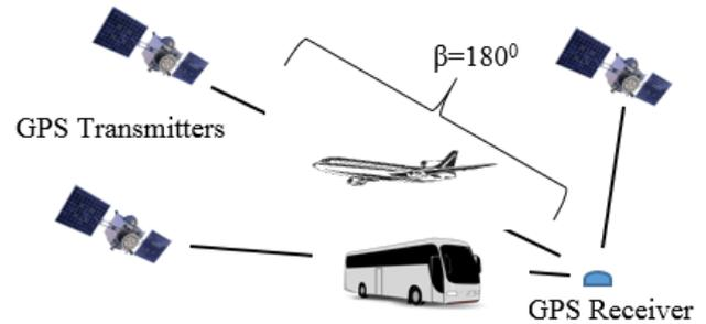
Fig. 1. Topology of Forward Scattering GPS system ( $\beta=180^\circ$ )
