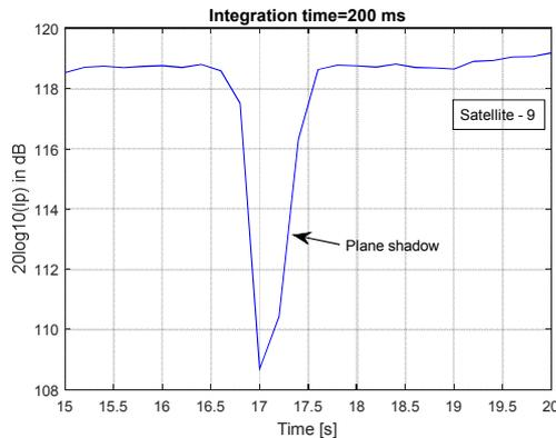
Fig. 8. Integrated satellite signal when crossing an airplane (Plane shadow)
