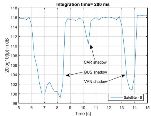
Fig. 5. Signal (shadow) from satellite 6
