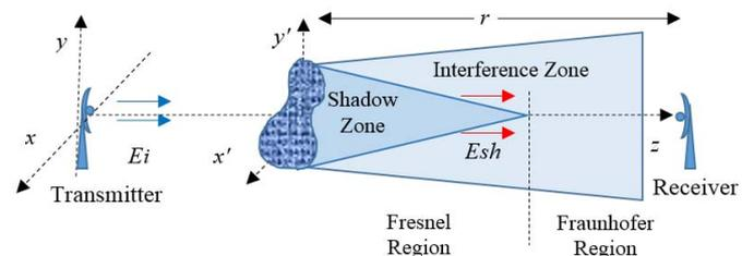
Fig. 2. Geometry of measuring of shadow radiation by an object sitting on the baseline, between transmitter and receiver
