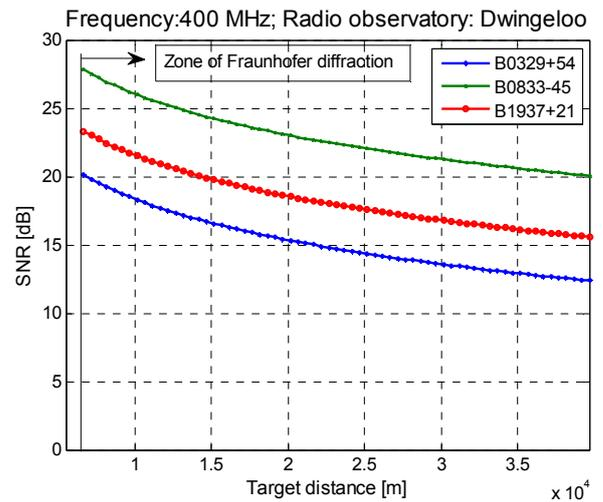
Fig.4: SNR vs. Rt ( $f=400$  MHz)
