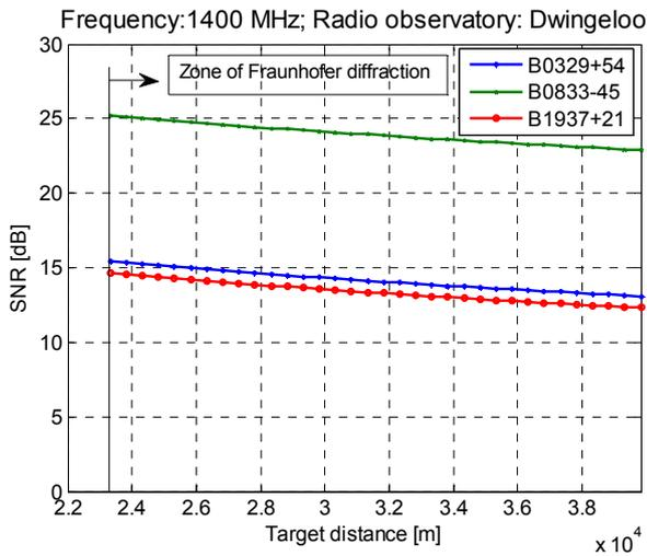
Fig.5: SNR vs.  $R_t$  ( $f=1400$  MHz)
