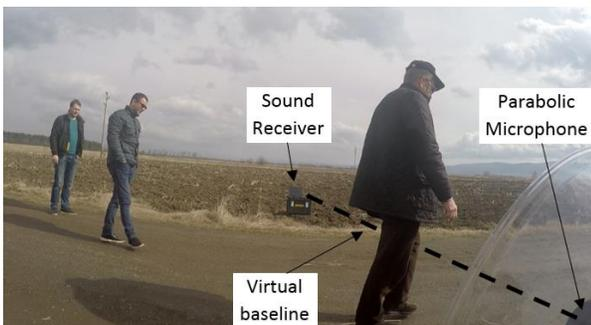
Figure 5: Sound recording system.
