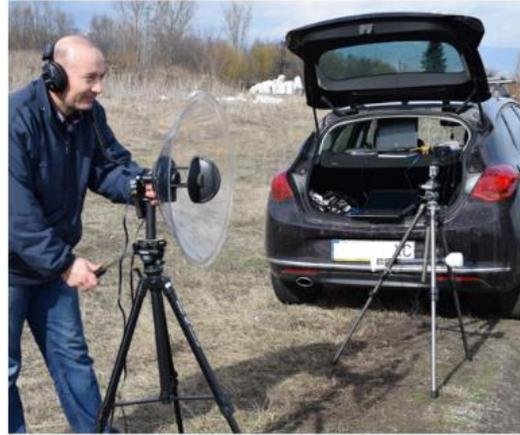
Figure 6: Wildtronics parabolic microphone.
