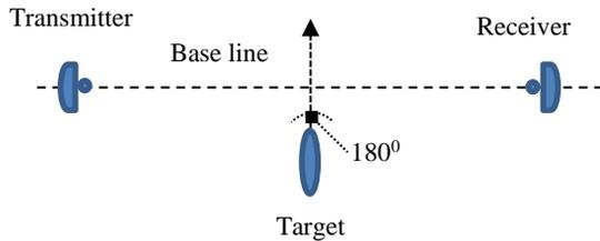
Figure 1: Illustration for forward scattering configuration.
