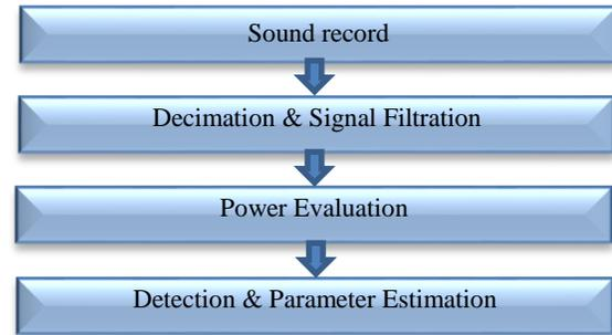
Figure 3: Blok-scheme of signal processing.
