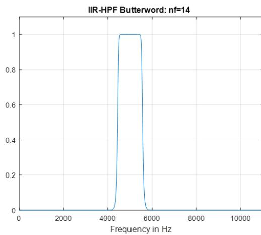
Figure 10: Frequency response of the bandpass filter.
