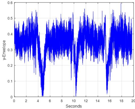
Figure 8: Envelope of sound signal (5 KHz).
