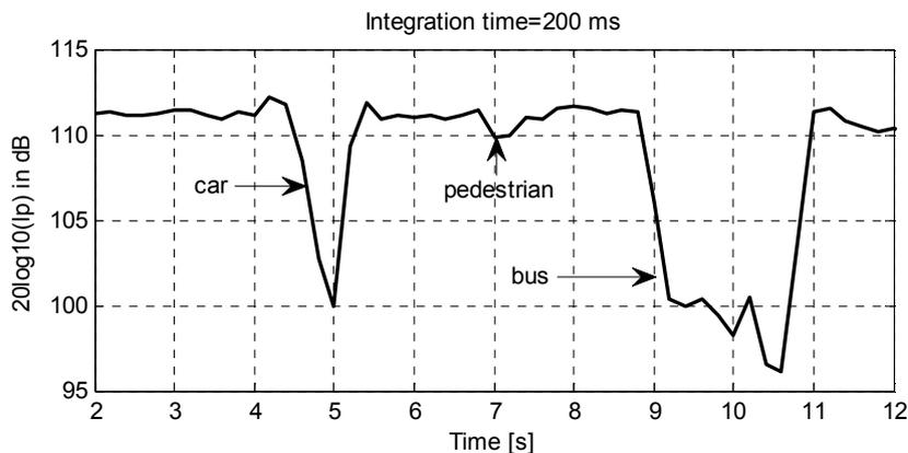
Figure 7: GPS radio shadows from car, pedestrian and bus
