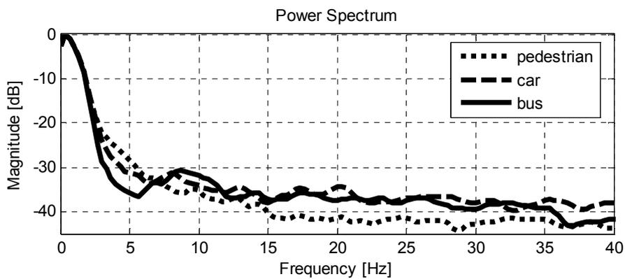
Figure 10: Power spectrum of pedestrian, car and bus
