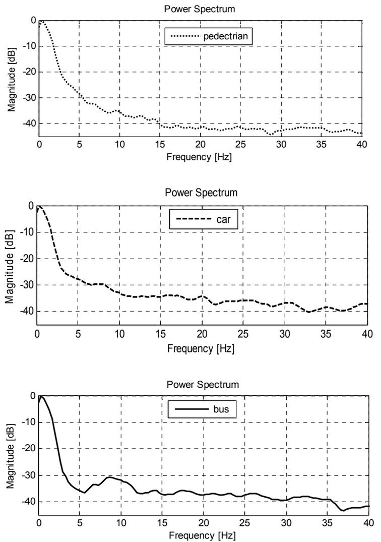
Figure 9: Power spectrum of pedestrian, car and bus
