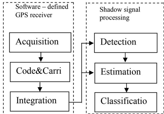
Figure 3: The general block-scheme of signal processing for target detection, parameter estimation and classification used in a passive GPS based FSR system
