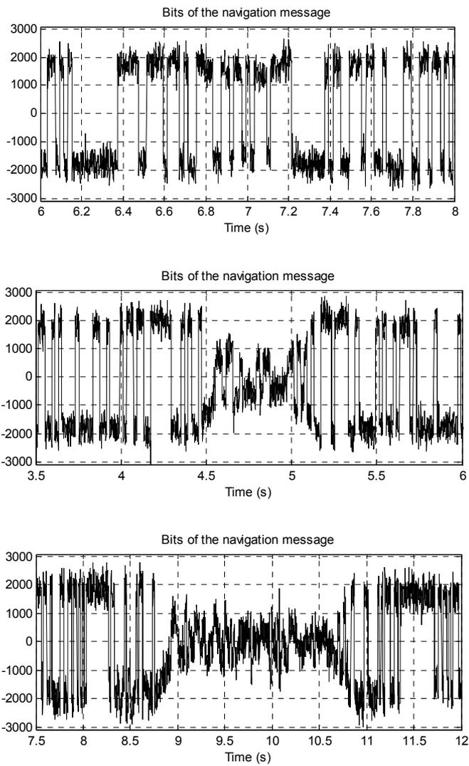
Figure 8: Bits of the navigation message (pedestrian, car and bus)
