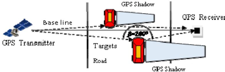
Figure 1: GPS FSR topology
