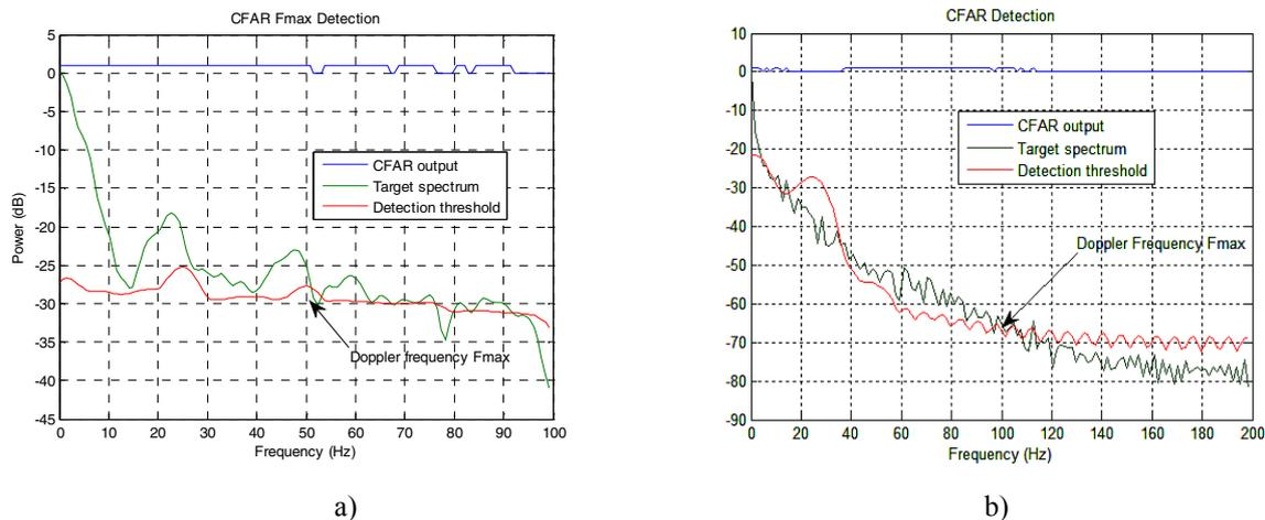
Figure 1 .Signal spectrum after MTI CA CFAR K/M-L detector. a) MISL boat, b) big boat
