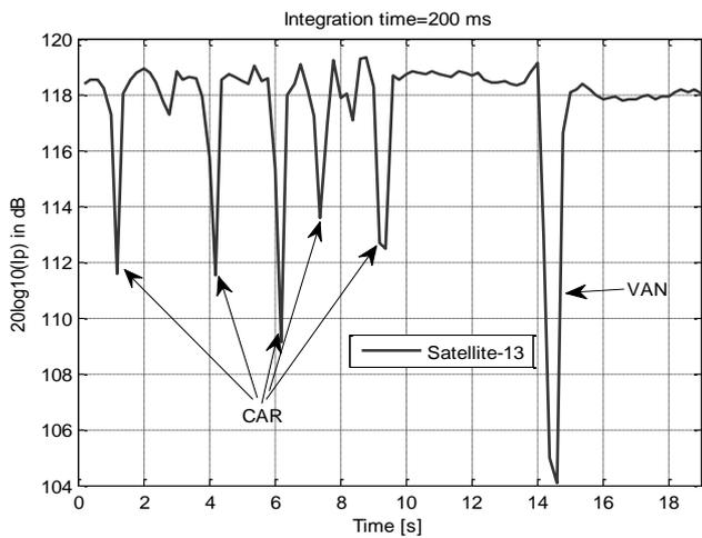
Figure 8. Filtered signals from satellite 13 (five cars and van)
