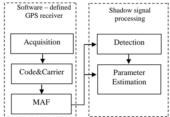
Figure 3. The general block-scheme of signal processing in a FS GPS system
