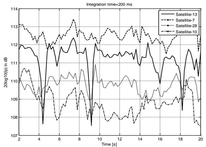
Figure 6. Filtered signals from satellites 7, 10, 13 and 28
