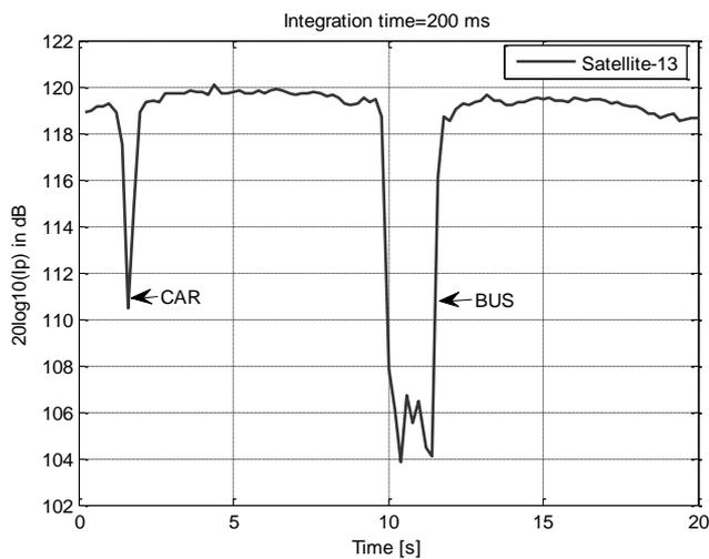
Figure 9. Filtered signals from satellite 13 (car and bus)
